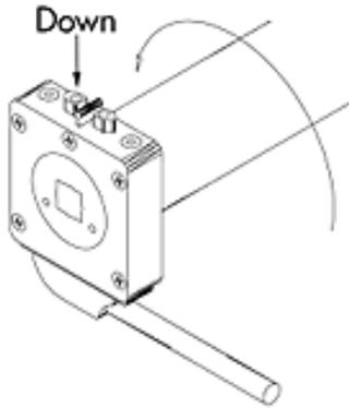
Move the shutter approx. 2 feet down and then up again in order to check the set position. If you missed the correct position in the "up" direction, let the shutter go to the correct position and press in the adjustment switch for the axle direction "Up". Now the exact position is set.
