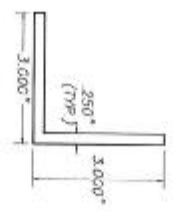
E 3x3x1/4" INSIDE MOUNT ANGLE 6061-T6 ALUMINUM ALLOY SCALE: 3/8" = 1"
