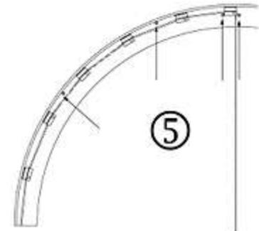
**Step 8.** Now the tension cord must be attached to the base slat. Run the tension cord down to the base slat from the center of the arch and insert into the predrilled hole located in the center of the base slat as shown in figure (6) Fish the tension cord through the base slat and tie a secure double knot on the end of the tension cord.
