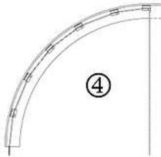
**Step 4.** Fish the tension cord into the guiderail through the 1x1 square channel of the guiderail. At the top of the guiderail, the tension cord must ride on the groove of the cord guide. Run the tension cord over top of the cord guide in the Guiderail (3) and let the end of the tension cord hang out.
