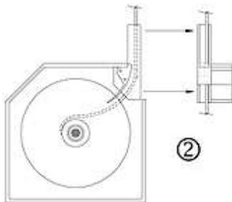
**Step 2.** Locate the guiderails. NOTICE: Each of the two guiderails are different from one another. Having a single cord guide at the top of the guiderail (1) can identify the guiderail that will be installed on the pulley side of the shutter; the guiderail to be installed on the motor side of the shutter does not have a pulley installed in it.
